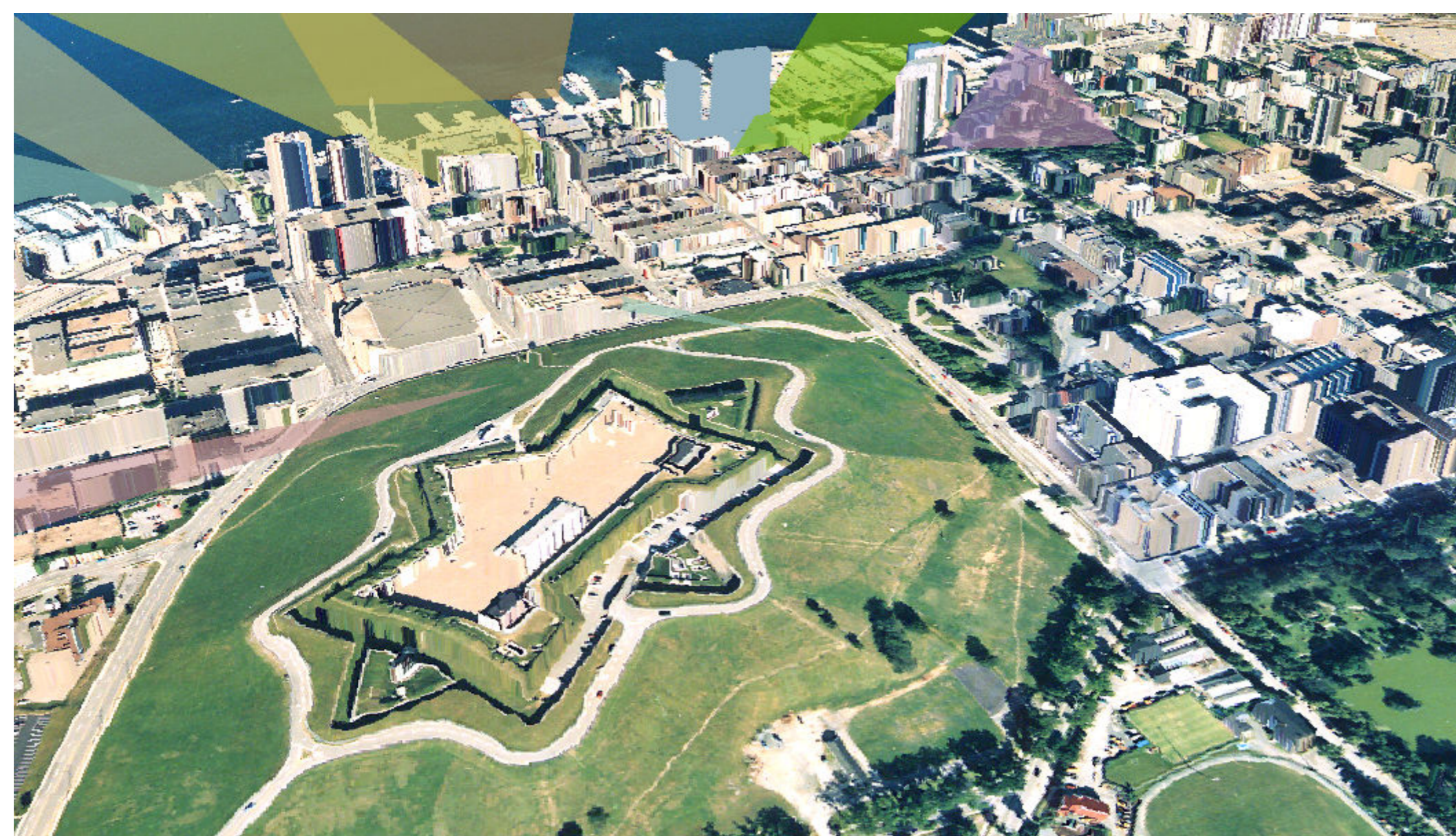
View Planes R6 (green) and C2 (blue) can be seen from this 3D rendering of Citadel Hill and the Proposed "Twisted Sisters" development (aqua blue building in the distance). This image was created by draping a georeferenced airphoto over a hillshade of Halifax produced with 3D Analyst using the lidar points and then viewed in Arc Scene. Although the resulting image is not of the highest quality it does highlight the capabilities of Lidar.
