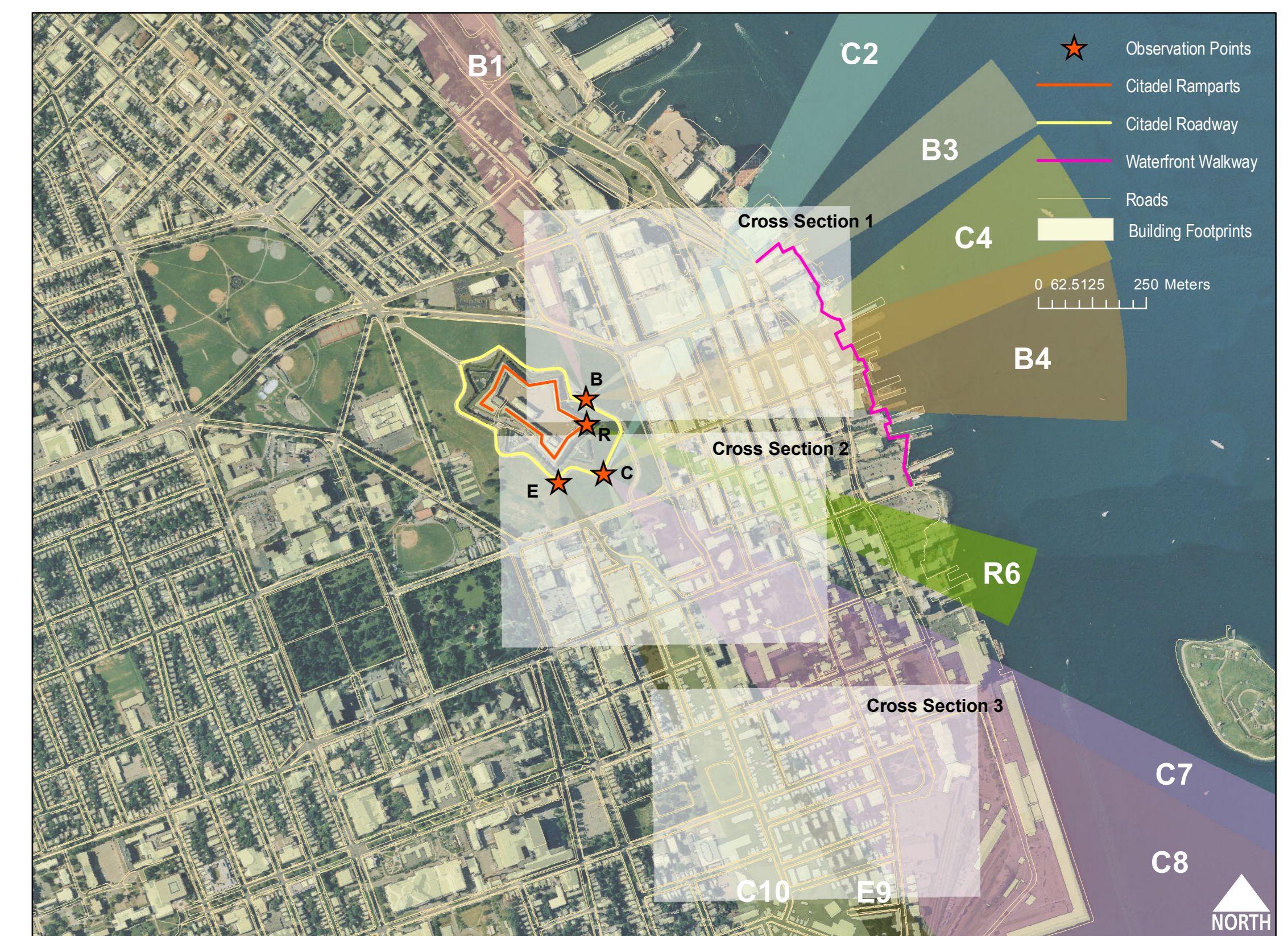
A georeferenced airphoto of Halifax which depicts the 10 viewplanes. The viewplanes were created in ArcGIS 9.3 using COGO with the coordinates, distances and elevations in the chart below. The viewplanes were then converted to points using the Feature Vertices to Point command and adding a field to the attribute tables called elevation. Then the points were used to create a tin for each viewplane using 3D Analyst.
